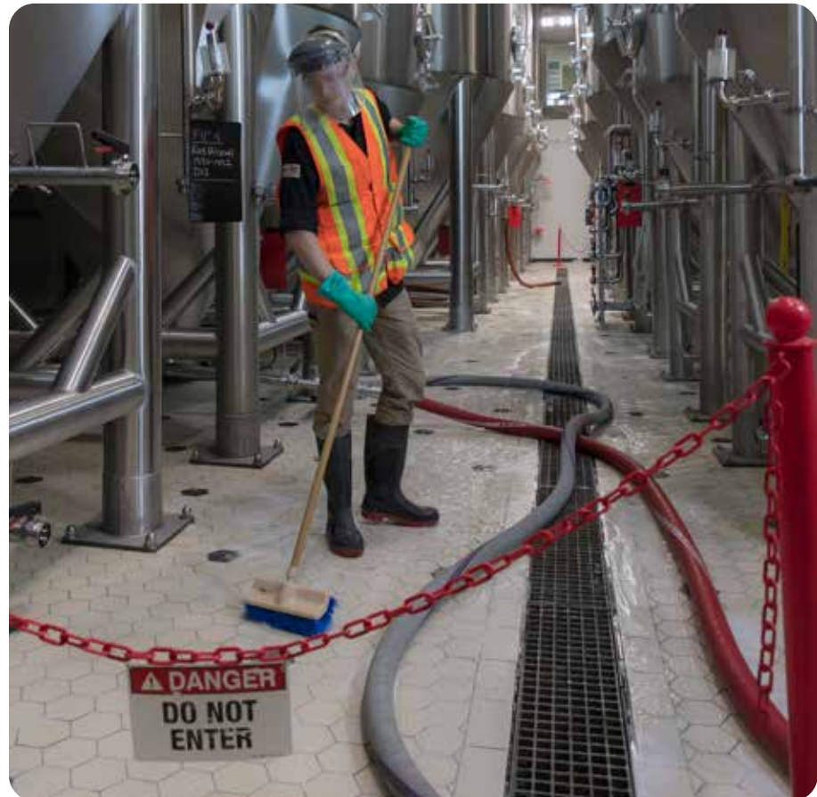
Restrict access to areas where hoses are on the ground.
